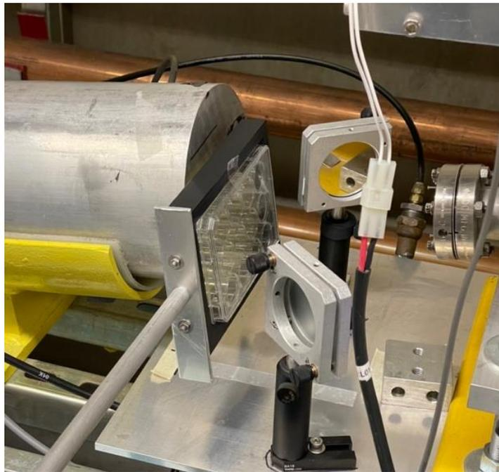
**Figure 18: Image of well plate set up in HIGS 5 experiment. A 2D translational stage holds the plate at approximately 15 cm distance from the exit window.**
